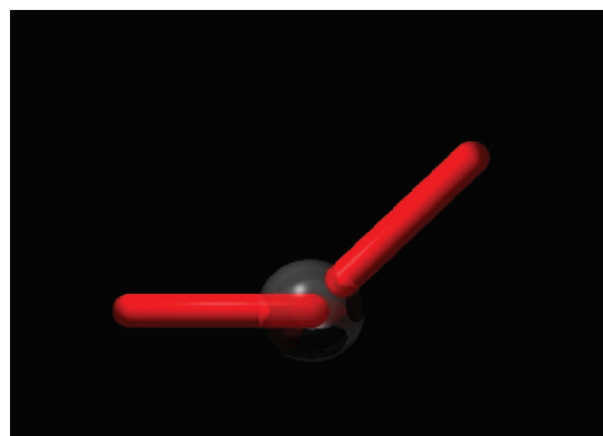
Figure 4. A sphere of interaction (SOI), represented by the transparent sphere, centered on one end of a terminal sphere of a spherocylindrical nanorod. Here, the radius r^* of the SOI is 2b , where b is the diameter of the nanorod. A close encounter occurs when the end of an approaching nanorod enters this SOI.
